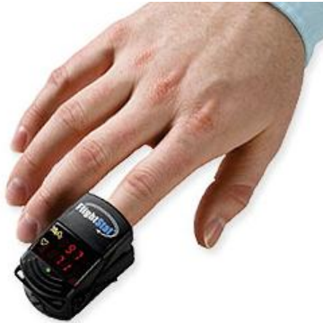
Figure 21 –Finger Orientation For The FlightStat
