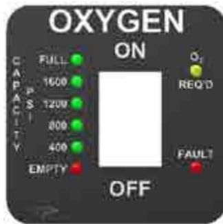
Figure 2 – Oxygen Control Panel
