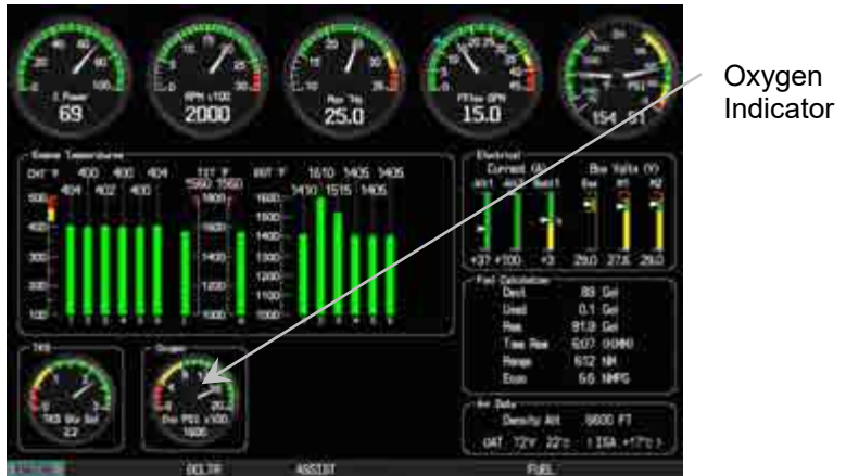
Figure 4 – Typical Cirrus Perspective MFD Engine Page
