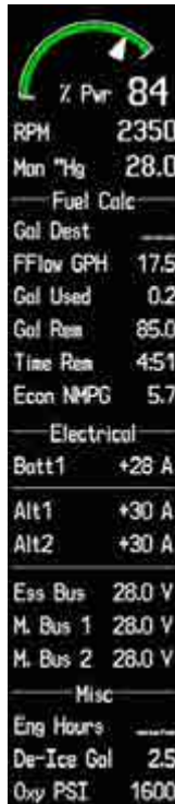
Figure 6 – Oxygen Quantity as shown on the Reversionary Mode System Display Page
