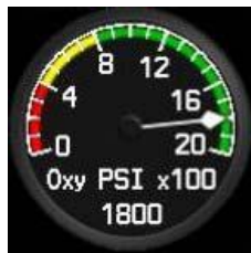
Figure 5 - MFD Oxygen Pressure Indicator Detail as Shown on Cirrus Perspective MFD Engine Page
