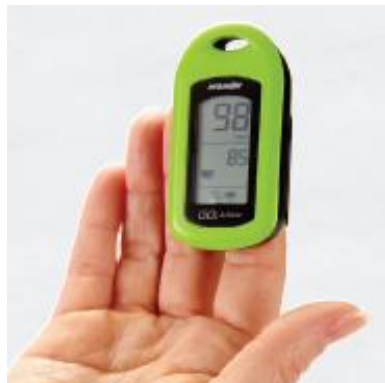
Figure 23 –Finger Orientation For The GO 2 Achieve
