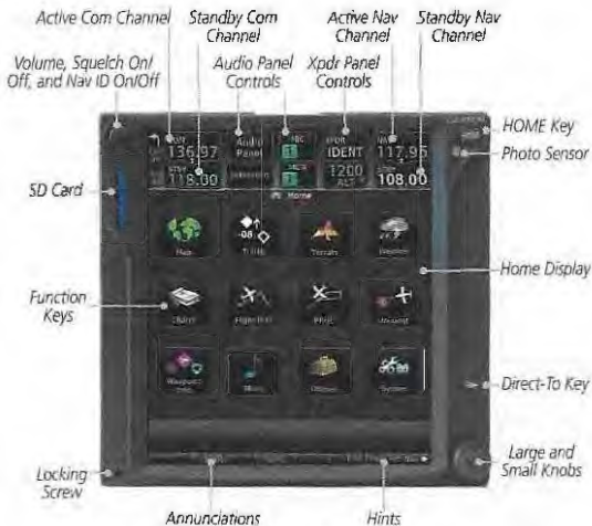
Figure 1 - GTN 750 Control and Display Layout
