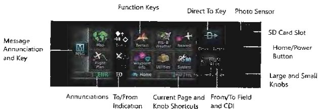
Figure 2 - GPS 175 Control and Display Layout
